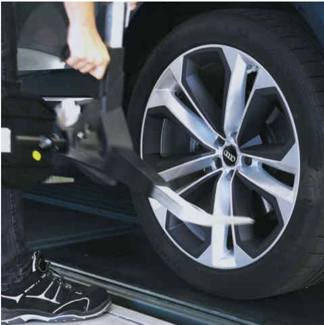
Q.Grip: Fast mounting without contact to the rim
